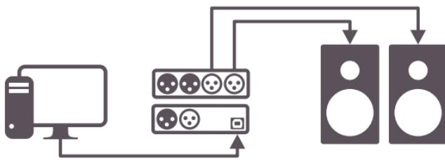
Connection of an analog mixing console
