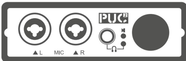
The combo jacks for the analog inputs allow the optional feeding of microphone or line level sources. They are both balanced.
