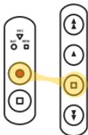
Press and hold the RECORD Button and simultaneously press the STOP Button on the Playback Keypad.
