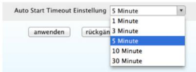
The timer indicates the timespan after that the card will be deactivated if your device does not access it. To restart WLAN function simply restart your device with FlashAir™ card inserted.
