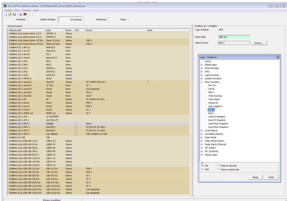
The GPO is to be active whenever the fader assigned to "MIC1" (and/or "MIC2") is open.
