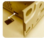
Rename your current firmware file ("intelli-8.1-x.x.fw8") to "fw.fw6" and duplicate it to the SD-Card ("Replace file" -> "Yes"). Disconnect the card from your PC ("Safely remove hardware") and put it back inside your Base Unit's card slot with the contacts pointing upwards. If you turn on your Intellimix, the rest of the update is executed automatically. This will take around 2 minutes.
