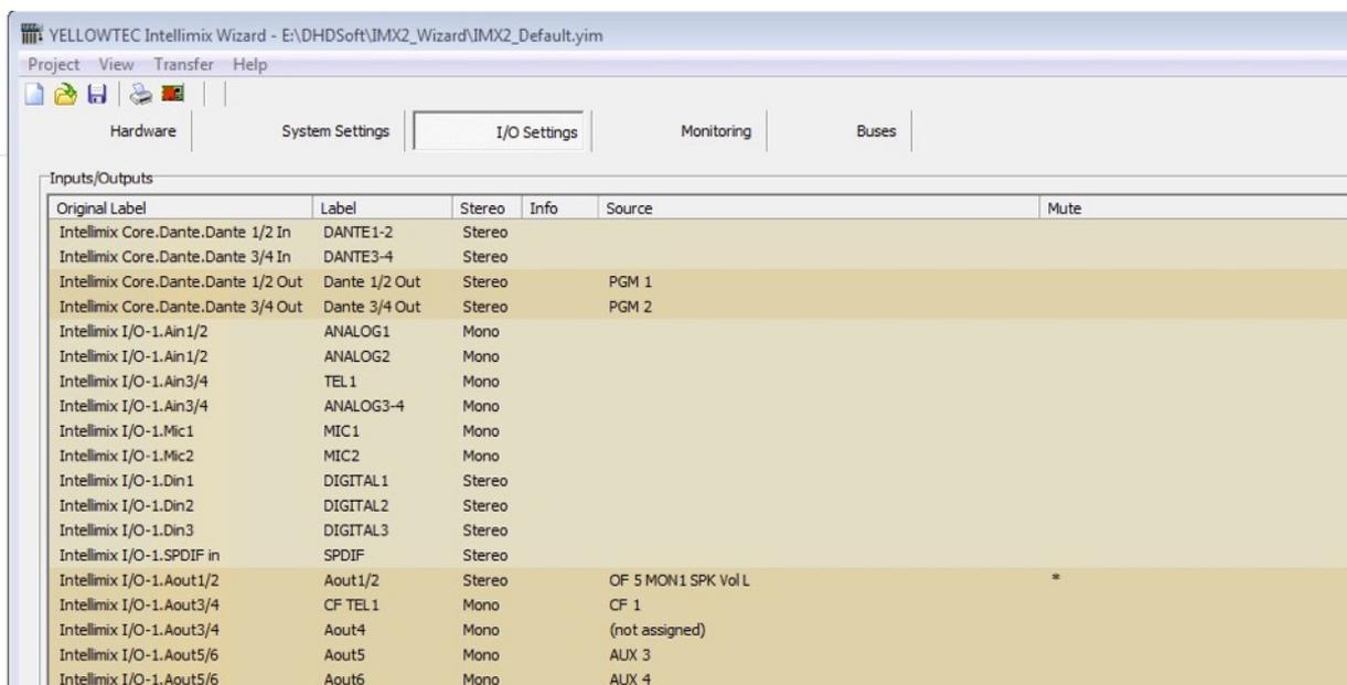
Choose the list entry with the original label “Intellimix I/O-1.Ain3/4”. These are the cinch inputs 3 (left) and 4 (right). In the right part of the screen adjustable options will pop up.
