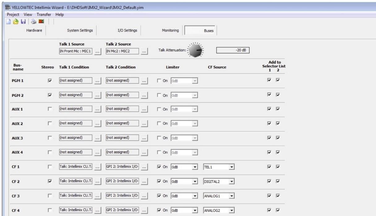
In the column “CF Source” choose “TEL1”. If this item does not appear in the list, the source is already assigned to another CF. In this case delete “TEL1’s” assignment to another CF and reassign “TEL1” to “CF1”.
