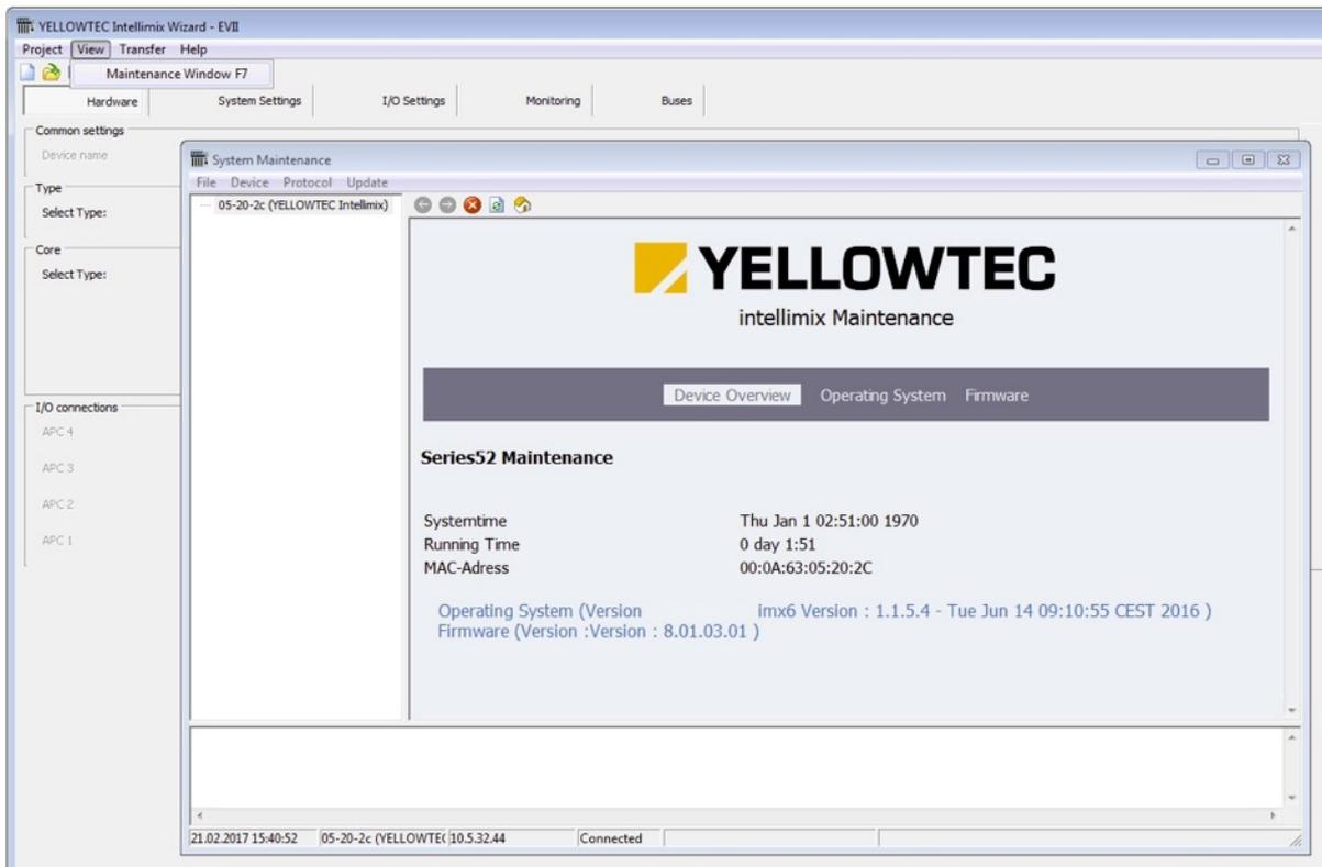
To change the network settings, please choose the menu “Device / Network Config...”. In the corresponding dialog window you can find fields consisting of information which can be partly modified. Serial numbers for example cannot be modified while the hardware name can.
