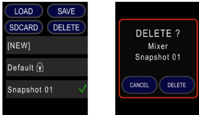
**REMARK:** The snapshots are in an alphanumeric order. Snapshots marked with the “LOCK” symbol are write / delete protected by the Administrator or System
