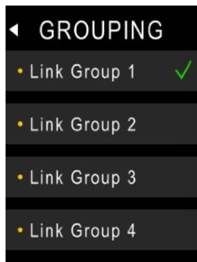
Linked faders move with the same dB offset. Moving one fader from the group makes the touched fader become the “Master”. All other faders in the group follow the master. To make the currently touched fader independent, simply press the SHIFT button.
