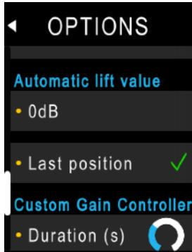
**0dB:** The fader moves to 0dB when opened, to -infinite when closed (default on previous firmwares)
